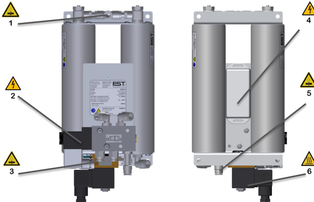
Fig 2: Dangers on the dryer
